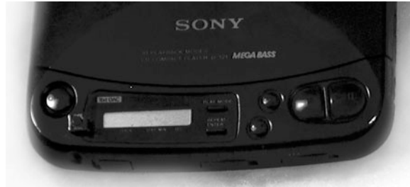
Figure 3: Detail of modified Sony D121. The small switch to left of display cuts the speed in half.
