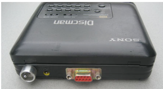
Figure 4: Modified Sony DT66 (my favorite player, quite rare), showing switch for mute enable/disable, and D9 connector for controlling player from a computer.
