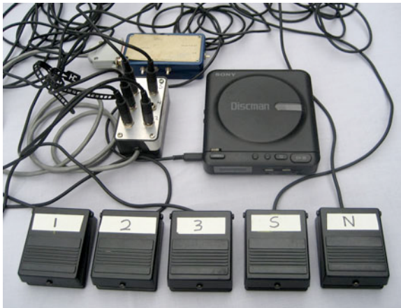
Figure 3: Set-up for Broken Light , showing hacked Sony D2 Discman; modified Sony remote control (in blue box); breakout box for connecting footswitches to remote control; footswitches to call up tracks for three movements (“1”, “2”, “3”), scratch across CD (“S”), and nudge through tracks (“N”).
