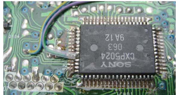
Figure 2: Lifted "mute" pin on chip in Sony D2 Discman (wires go to switch for mute enable/disable.)
