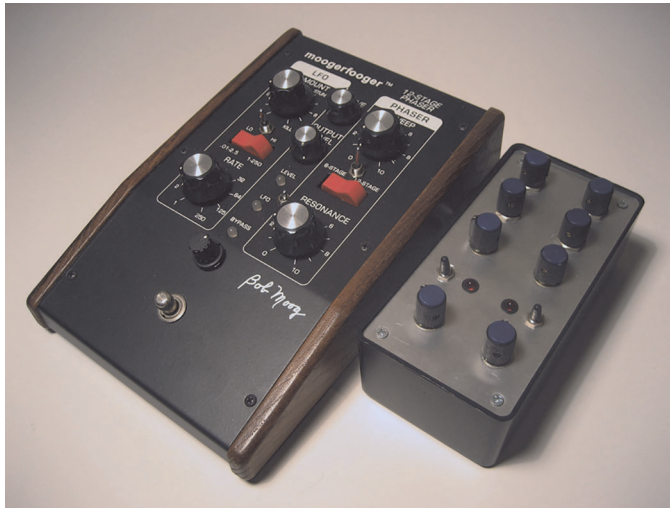
FIGURE 7. Modified Moogerfooger M103 Phase Shifter (box on right contains envelope followers), Nicolas Collins (2001).
