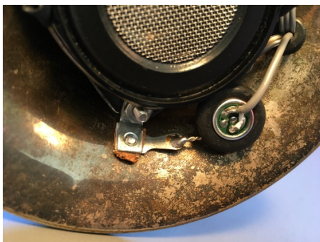
Figure 25: pressure-zone electret microphone mounted inside bell
