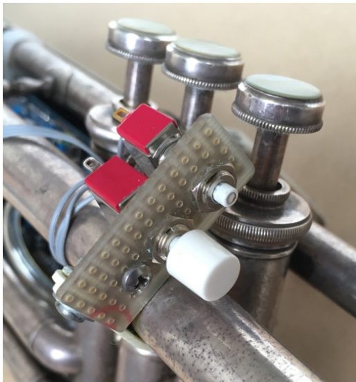
Figure 10: switches near top of valves
