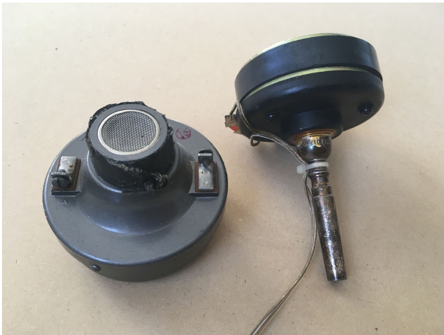
Figure 2: Drivers used for saxophone (left) and trombone (right), 1975.
