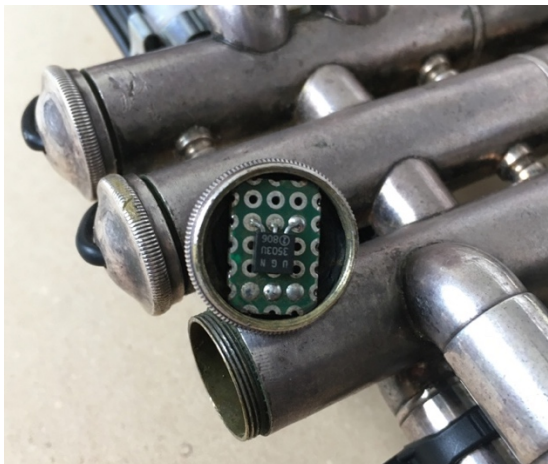
Figure 8: valve sensor: Hall effect sensor (left), and magnet embedded in valve base (right)
