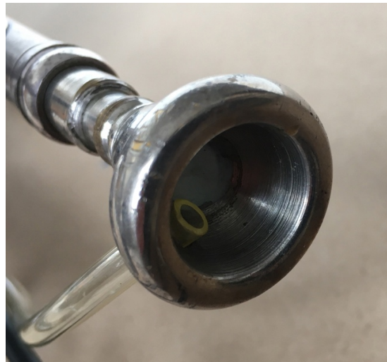
Figure 9: air pressure sensor and hose coupling to mouthpiece
