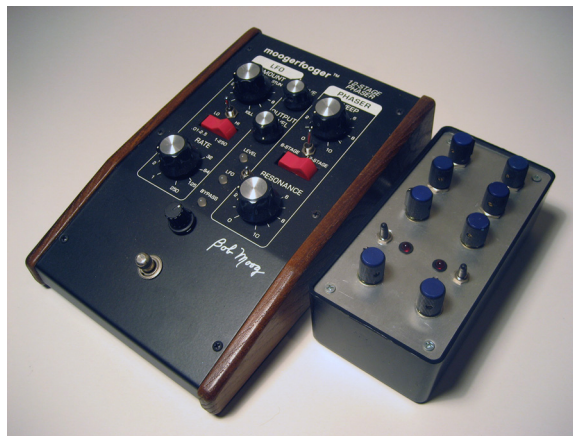
Figure 6: Modified Moogerfooger M103 Phase Shifter (box on right contains envelope followers), Nicolas Collins (2001)
