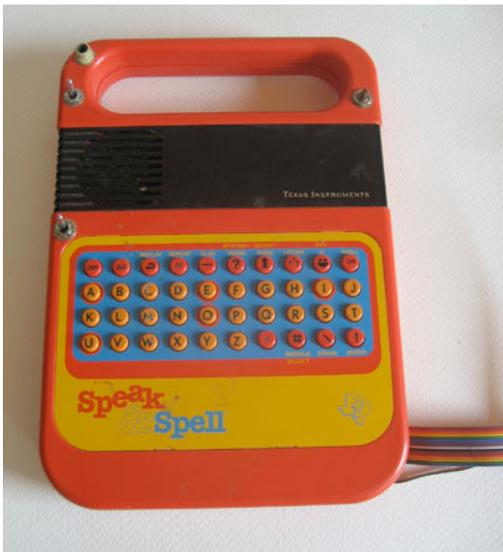
**Figure 6:** *Speak and Spell* modified to function as a computer speech synthesizer.
