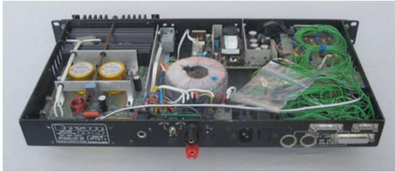
**Figure 11:** Trombone-propelled electronics rev. 2: open Bryston chassis (rear view) showing amplifier channel on left, SensorLab circuit boards on right.
