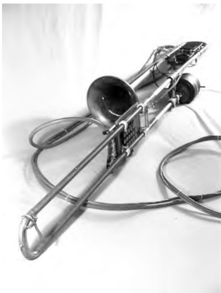
Figure 3: Trombone showing keypad, speaker, tip of breath control visible behind speaker.
