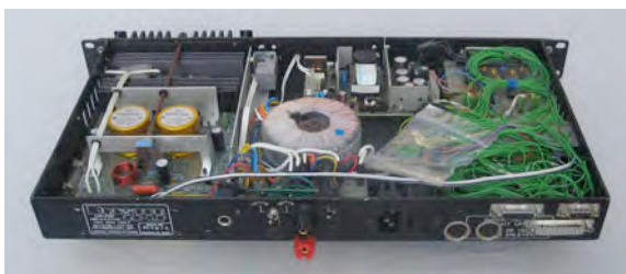
Figure 10: Open Bryston chassis, rear view, showing amplifier channel on left, SensorLab circuit boards on right.
