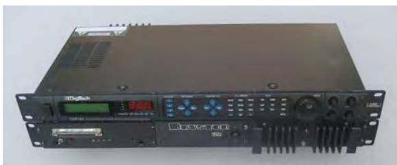
Figure 9: Trombone-propelled electronics rev. 2: Digitech TSR-24S above; Bryston 2B-LP chassis below, containing amplifier channel for trombone speaker in right side, re-packaged STEIM SensorLab in left.
