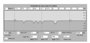
This picture shows the bass response boosted, and the highs rolled off. The number boxes under either end of the graphic display indicate the corner **frequency** of each filter, while the amount of boost and cut are referenced to the dB scale at the right end of the display. The shelving EQ can be reset to flat by clicking the button marked **flatten shelving**.
