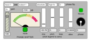
These panels are responsible for the moment-tomoment behavior of the feedback; each one emulates a *Countryman Phase Shifter*. The primary function of each **PHASE SHIFTER** is to insert a very short, phase-dependent audio delay into the audio path. This delay is controlled by the *loudness* (and optionally the *pitch*) of the audio signal: in emulation of a nervous sound engineer who jerks the mike
