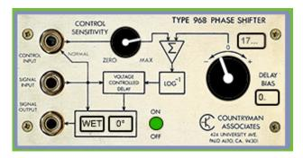
By inserting a very short frequency-dependent delay in the audio signal path the Countryman emulates changing the distance between the microphone and the speaker, which causes the feedback to jump to another pitch. *Pea Soup* increases the amount of delay in proportion to the loudness of the feedback, to create a self-stabilizing system by applying <u>negative</u> feedback to control <u>positive</u> feedback.
