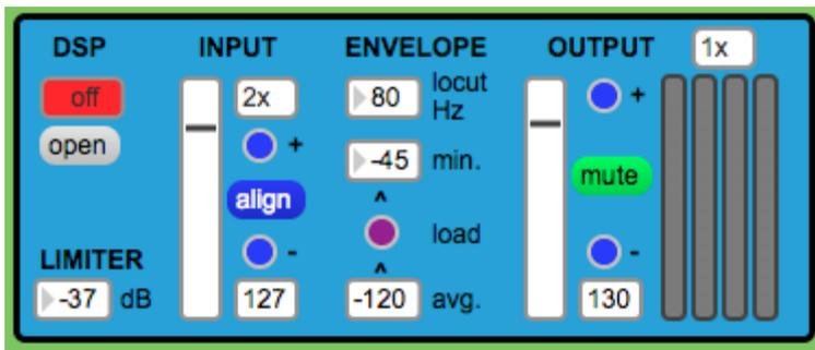
At the top left of the window are two controls for the **DSP** that processes audio signals. The topmost pull-down menu (default state **off**) turns on the DSP for only the *Pea Soup* patch (**soup**) or all Max audio patches currently open (**all**). Select either **soup** or **all** to run *Pea Soup* (it doesn't matter which.)
