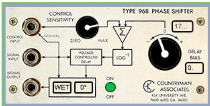
By inserting a very short frequency-dependent delay in the audio signal path the Countryman emulates changing the distance between the microphone and the speaker, which causes the feedback to jump to another pitch. *Pea Soup* increases the amount of delay in proportion to the loudness of the feedback, to create a self-stabilizing system by applying negative feedback to control positive feedback.
