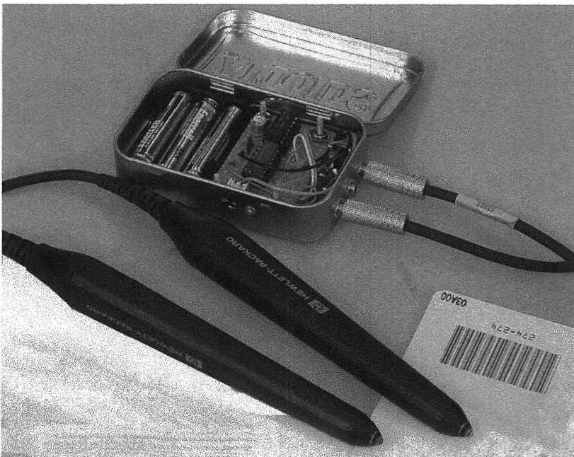
Figure 24.17 Bar code readers with power supply and planning circuit (Nicolas Collins).
