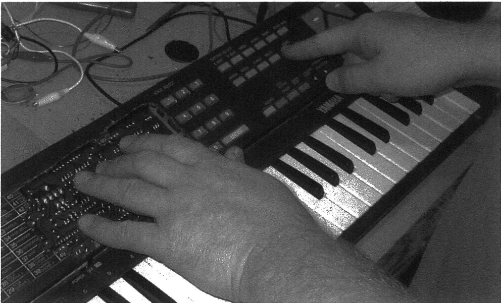
Figure 15.16 Mike Challis (UK) playing his hacked Yamaha PS-140 by touching circuit board directly through a hole cut into the case.
