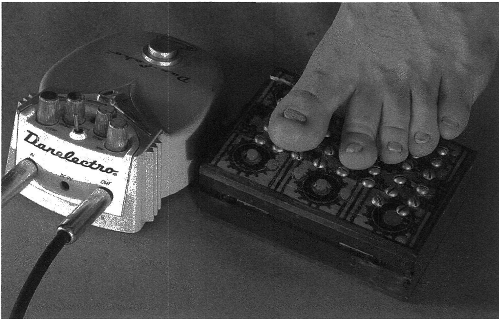
Figure 15.18 Hacked guitar effect pedal by Chris Powers (US), with electrode contacts for toes.
